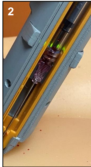
2 Blood-sensing circuit activated
