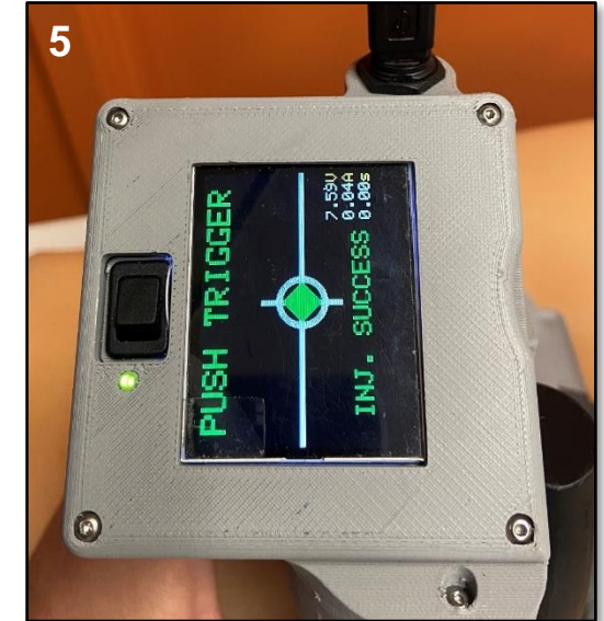
5 Blood flashback confirmed • Drive motor stops • Operator notified
