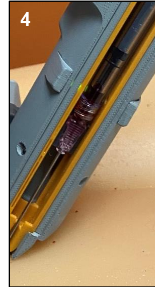
4 Blood drawn into syringe, blocking light and tripping blood-sensing circuit
